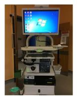
The EndoRAAD PC can be placed on a separate trolley which can be moved with but independently of the Endoscopic Camera Stack. The associated image capture cabling between the two is configured with a robust twist and lock connector for ease of movement.
