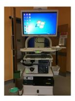
The EndoRAAD PC can be placed on a separate trolley which can be moved with but independently of the Endoscopic Camera Stack. The associated image capture cabling between the two is configured with a robust twist and lock connector for ease of movement.
